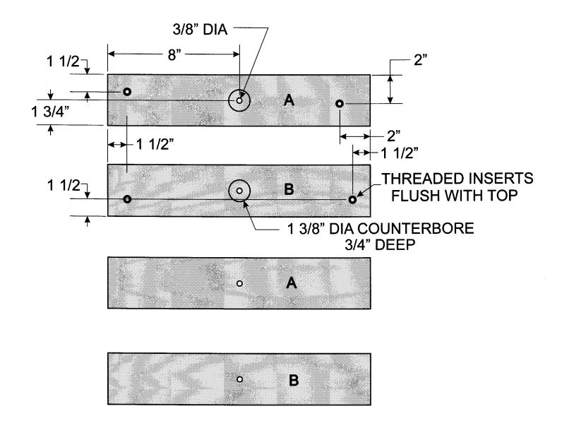
DRILL 3/8" DIA HOLES THRU "A" BOARDS AT THE SAME TIME, MARKING TOPS AND OUTSIDE EDGES TO ENSURE PROPER ALIGNMENT DURING ASSEMBLY. REPEAT WITH "B"s.
